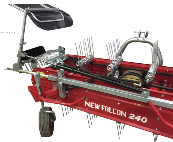
Fig. 3 Dettaglio supportino e boccole in materiale autolubrificante Belt with double-rod connecting bars detail in auto-lubricating material
