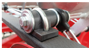
Fig. 3 Dettaglio supportino e boccole in materiale autolubrificante Belt with double-rod connecting bars detail in auto-lubricating material
